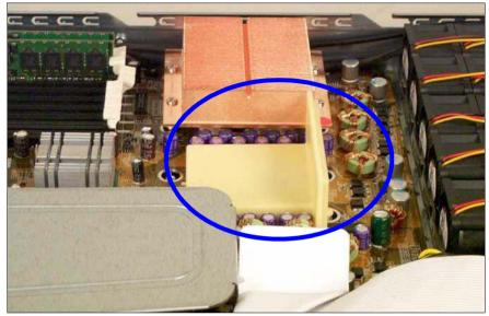
Figure 7: Removing the heat sink dummy
